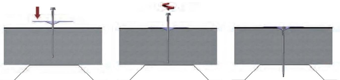
1. Position the pressure plate and insert the fixing.
