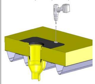
8). Install the Armourplan or Spectraplan membrane by hot air welding to the top of the appropriate membrane flange connected to the extension unit.
