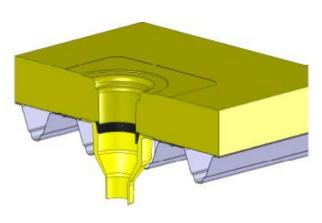
7). Install the extension unit by pushing through in to the rubber sealing ring and secure by fixing the membrane flange to the substrate using IKOfix fasteners and IKOfix GOK thermally broken pressure plates.
