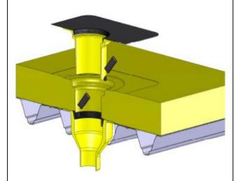
6). Shorten the extension unit if necessary and apply the enclosed lubricant to the rubber sealing ring and the bottom of the extension unit. The extension unit should go past the bottom of the rubber sealing ring to ensure a good fit.
