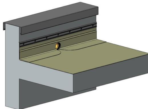
5). The Easy Flow dome grate can be inserted into the outlet if necessary.
