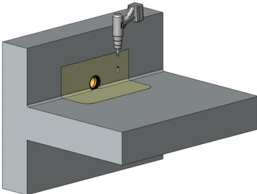
4). Hot air weld the roof membrane to the Easy Flow membrane flange.
