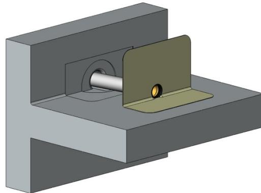
3). Secure the flange of the Easy Flow mechanically using IKOfix fasteners and pressure plates.
