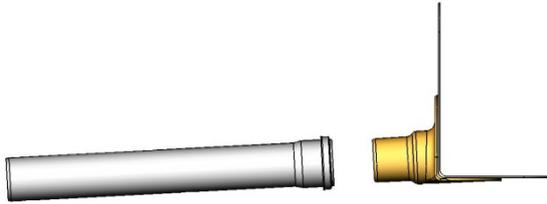
2). Push the Easy Flow outlet with connected connection pipe through the core drill into the parapet.
